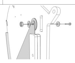
Fit the Small Clevis Pin into the hole in the Metal Door from behind, and secure it using a washer and split ring. This can be a little awkward. We find that holding the split ring open by inserting a flat-bladed screwdriver between the rings can make this task easier. But please mind your fingers!
