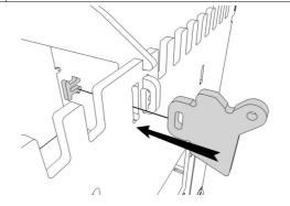
Fit both Side Walls to the Lower Back Wall and Base using Pi Clips. Ensure that the Double-hole lugs are at the front. Then fit the Roof Support using Pi Clips.
