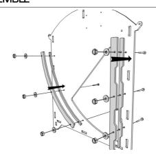
1 Fit two Vent Covers to the patterned face of the Right Side Wall each using an M6x30mm screw, a standard washer, a 25mm washer and a nylock nut. Tighten the nuts until the vents can rotate using gentle pressure. They should not spin freely.
