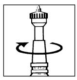
Insert the black valve unit into the top of the cone, valve downwards. Before inserting the valve into the top of the cone, check to ensure the top and bottom caps (part nos 412767
