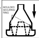
round when the assembly is viewed from the underside. Finally, place the black chick saving ring into the trough of the cone if required for use with day old or very young stock.
