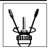
Place a nut, thread outwards, onto the end of the tube. Push Hanger Strap over filter top. Push the tube onto the tapered end of the filter top as far as it will go. Tighten the nut firmly. Repeat at the Saddle Connector end.
