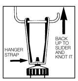
For the most efficient operation, it is necessary to suspend the Waterers above the height of the backs of the birds. With large birds and Layers the Waterers should be set at about their eye level.
