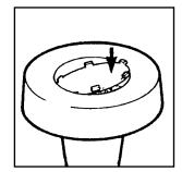
Remove all components from carton. Fill the recess in the underside of the black ballast bowl with ballast or sand, up to just below the holes at the top of the recess (3lbs or 1.36kilos). Place the ballast retaining lid (with six lugs uppermost) into the ballast recess, fitting two adjacent lugs into their recesses. Then press each of the remaining four lugs home working round in a clockwise direction.
