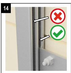
It must be in the second slot in each channel. The screws and nuts must be at the front.
