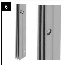
Locate the rivet in the hole, then push it in to secure it.
