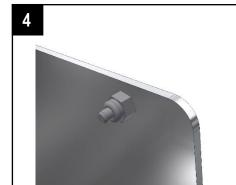
Tighten each nut by turning the screw with a screwdriver whilst holding the nut with pliers or a spanner.
