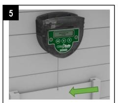
Tie the ChickSafe cord to the hole fitted with the grommet in the top of the door.
