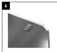
Tighten each nut by turning the screw with a screwdriver whilst holding the nut with pliers or a spanner.
