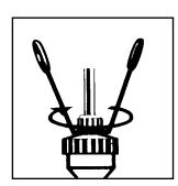
Place a nut, thread outwards, onto the end of the tube. Push Hanger Strap over filter top. Push the tube onto the tapered end of the filter top as far as it will go. Tighten the nut firmly. Repeat at the Saddle Connector end.
